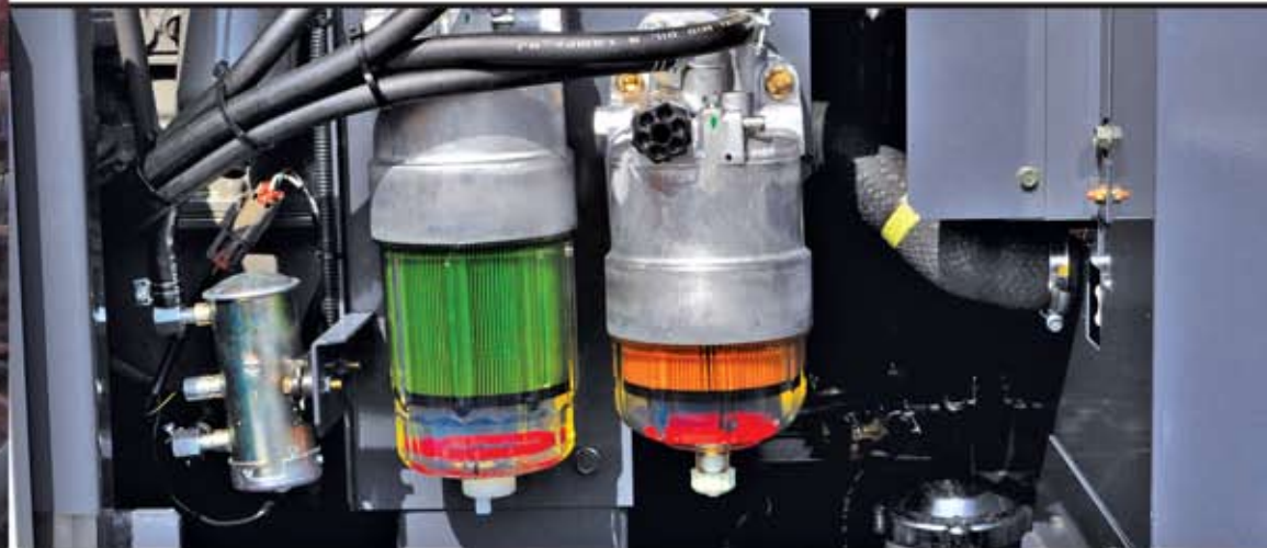
EFPA pump and dual acrylic "cartridge style" fuel filters.
